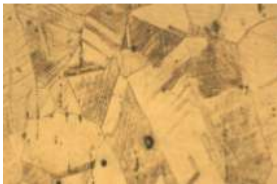
Figure 1. Optical Microstructure (x100) of AISI 316 L austenitic stainless steel in as received condition.
