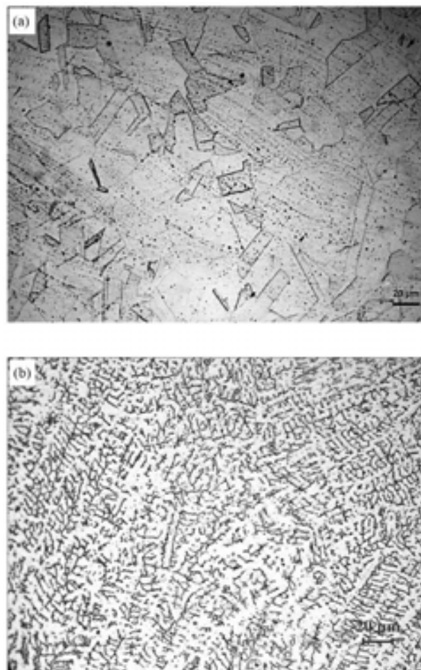
Figure 2. Optical micrographs of (a) as-received 190 sample and (b) weld metal tested at 25°C.
