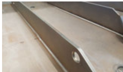
Figure 5: A finished & welded side walls with automation
