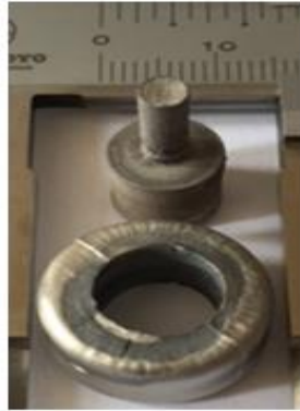
Figure 2. Sintered sample (with no interlayer) at 1200 °C for 240 min
