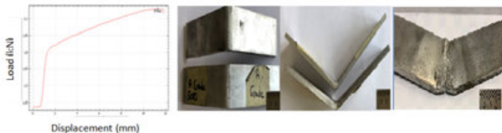
Figure 8. Three-point bending load-displacement curve and tested samples
