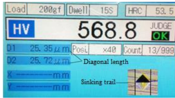
Figure 4. Micro hardness of nickel coating before sintering
