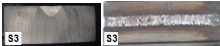
Figure 2. Macrographs of S3 sample FeCrC based composite coating.
