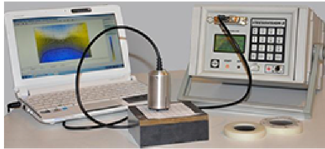
Figure 2. Indicator of Mechanical Stresses (IMS) consist of data collector, probe (transducer) and Laptop for process and store results
